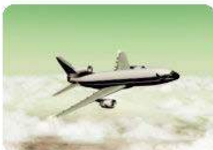
Fig (10) The horizontal component of the lifting force on the aeroplane acts as a centripetal force.
